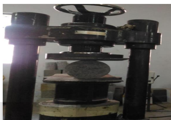
Split Tensile Strength Test on Cylinder
